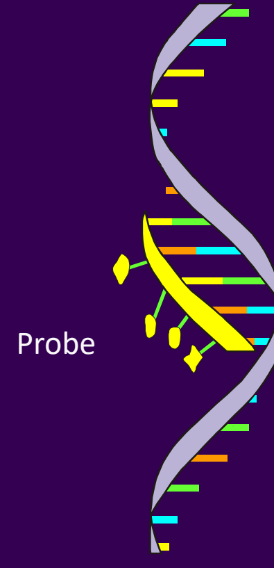
Probe binds to denatured DNA and emits a signal
